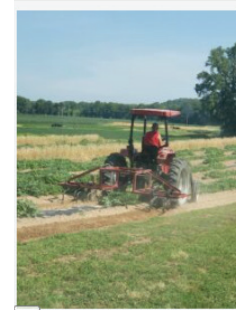
Figure 4. A tractor-mounted S-tine cultivator removes small weeds from row middles of plasticulture watermelon (Photo by J. Arana).
